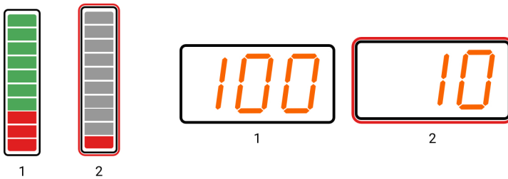
Figure 8. Scale of charge level of the energy storage device
